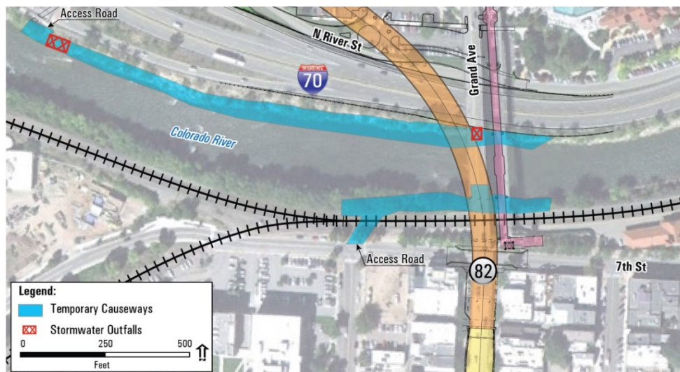
FIGURE 2-17. TEMPORARY CAUSEWAYS AND ACCESS ROADS
